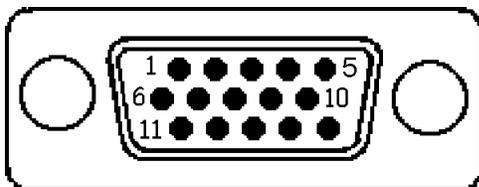
NOTES: I/O lines 1 & 2 each have internal 4.7kΩ pull-up resistors connected to the internal +5 VDC-100 mA power supply.
