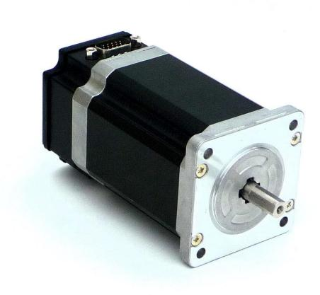
The 24 frame motor has a slightly larger cross section and a heavier shaft, but has the same mounting holes and pilot diameter as a NEMA 23 motor, for easy mounting. The 24 frame motor is designed to have a significant torque advantage over standard 23 frame motors due to the added rotor radius available.
